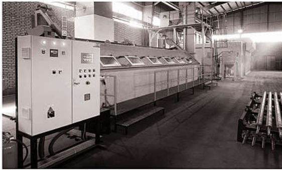
Fully automatic Sandblast with a working length of 7 meters
