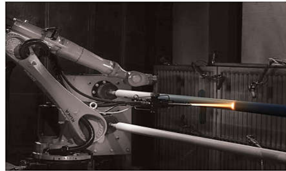
6 degrees of freedom robot with the ability to move on the rails (7th axis)
