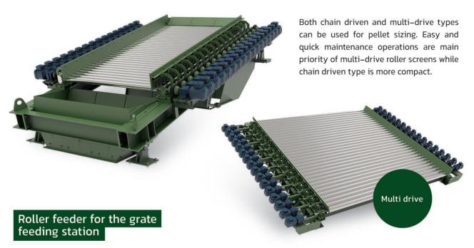
The roller feeder is placed at the grate feeding station. Pellets coming from the balling department are discharged on it. One of its purposes is to remove the fines coming from the breakage of pellets on their way to the furnace. Its main function is to distribute evenly the good pellets on the indurations furnace grate. This equipment can be driven with a chain or with individual drives. The roll length can be provided up to 6 meters upon feeding capacity.
